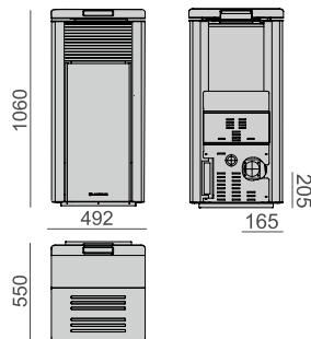
VERONICA AIR is a cubic style pellet stove. The facade has an integrated large tinted glass door offering an airtight tank with an 11 kW rated output.
